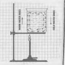
Heat is applied at the bottom. The heated material above the flame rises. Colder fluid sinks on the opposite side, then flows toward the candle side to replace the rising fluid. A "convection current" is formed. Later we will show how rising and sinking air currents are responsible for much of our weather both good and bad.
