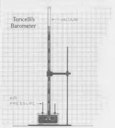
causing the mercury in the glass tube to rise. When the pressure was low, the mercury in the glass tube fell.
