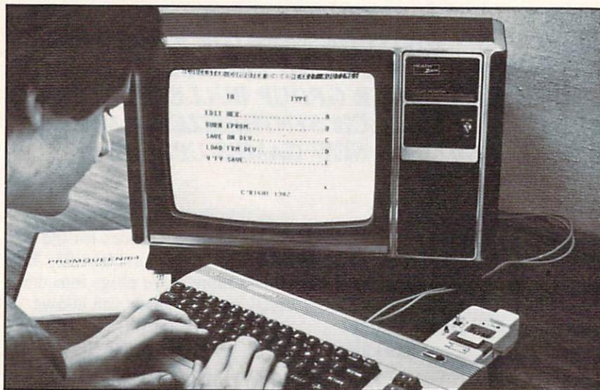
*The Promqueen/64 is inserted into the expansion slot.*
