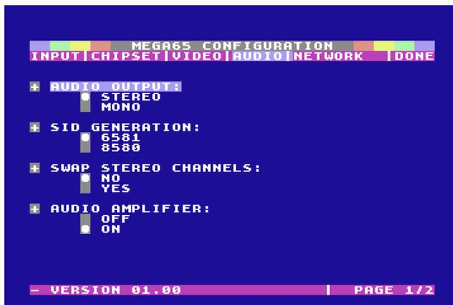
**Audio output** can be configured to use full stereo, or to send a monoaural signal to both speakers. When in stereo mode, various audio devices in the MEGA65 can be panned to the left or right using the audio mixer in the Freezer menu. The default settings pan the four SID chips slightly to the left and right.
