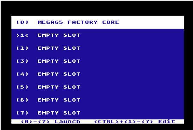
You can select a core to boot using the cursor keys and
