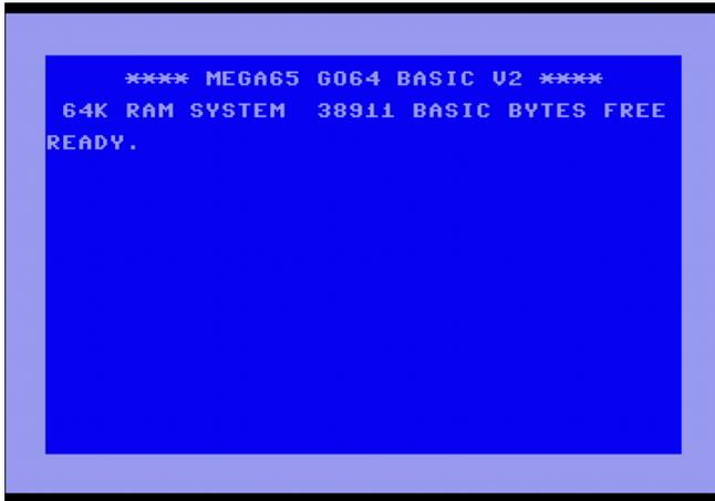
GO64 mode is actually just a temporary re-configuration of the MEGA65. All of the MEGA65's features are still present, including the Freezer menu for mounting D81 disk images.
