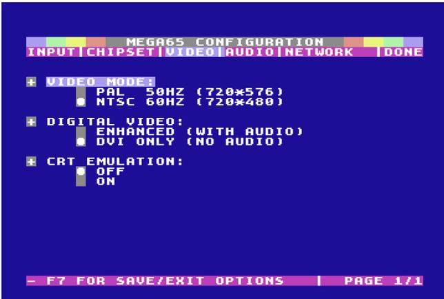
**Video mode** selects between the PAL compatibility mode and the NTSC compatibility mode. You can also change this while running programs using the Freezer menu.
