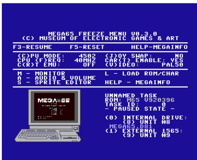
One feature to remember when playing games is the “(J)OY SWAP.” This causes the two joystick ports to trade numbers. If you have a joystick in port 2 and you start a game that expects a joystick in port 1, instead of disconnecting and reconnecting the joystick, open the Freezer menu, press **J** to swap the port numbers, then resume your game.
