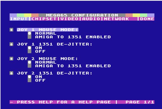
The MEGA65 supports the Commodore 1351 mouse, the Commodore Amiga mouse, or modern equivalents such as a USB mouse connected with a [mouSter](#) adapter. The port must be set to the correct mouse type, where **normal** refers to the 1351 mouse. If an Amiga mouse is connected while the port is in the **normal** mode, it may interfere with the behavior of the keyboard.
