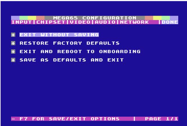
When you exit the Configuration Utility, you will be prompted to “power-cycle” the computer. Switch the computer off, then switch it on again.
