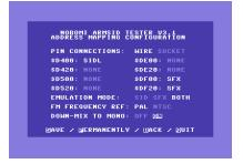
With this configuration you can play all OPL FM synth music for Sound Expander and one SID together. You can down-mix to mono, if you do not use stereo output on your C64. It is possible to switch to SFX only mode (without SID). In that case all computing power is put to the FM synthesis and SFX emulation is even better and goes to both channels.
