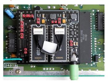
Configure ARM2SID with the provided ARMSID TESTER utility. Start it, choose \$D400 SID, select M for ADDRESS MAPPING CONFIGURATION and select PIN CONNECTION: SOCKET, then choose what to play in the LEFT and RIGHT socket. If your socket supports \$DFxx addressing, you can use SFX (FM) too.
