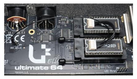
The SID A[5..9] brings an addition address line to the ARM2SID to recognize more different addresses where internal SIDs/SFX could be positioned. It is controlled by Ext DualSID Range Split setting of Ultimate 64 configuration.
