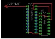
Shorten all pins on 74HCT541 with the exception of pins 10 and 17. Wire (solder) together all pins 2-10 and 11-18. Piggy back place 74HCT541 on top of U3 and solder the pin 10 of 74HCT541 to the pin 8 of U3. Then solder the pin 17 of 74HCT541 to the pin 15 of U3. Connect VCC (the pin 20 of 74HCT541 to the pin 16 of U3) and connect G2 (the pin 19 of 74HCT541 to the pin 14 of U3) by short wires. Finally connect 64/128 signal from the MMU pin 47 to the pin 1 of 74HCT541.
