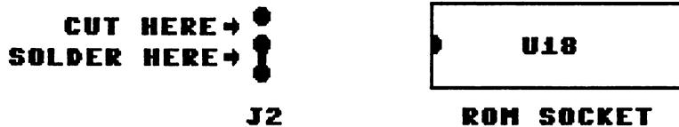
If the U1 controller in your REU is a rectangular chip, then the jumpers will be located near the connector end of the board. Two jumpers on this version of the REU must be connected. Connect the two pads between J5. Locate jumper J2. Connect the center pad of J2 with the pad to the left of center (labeled 27256). Refer to the illustration below. Replace the circuit board in the bottom of its plastic case and temporarily set the top cover back in place. Plug the REU back into the computer.
