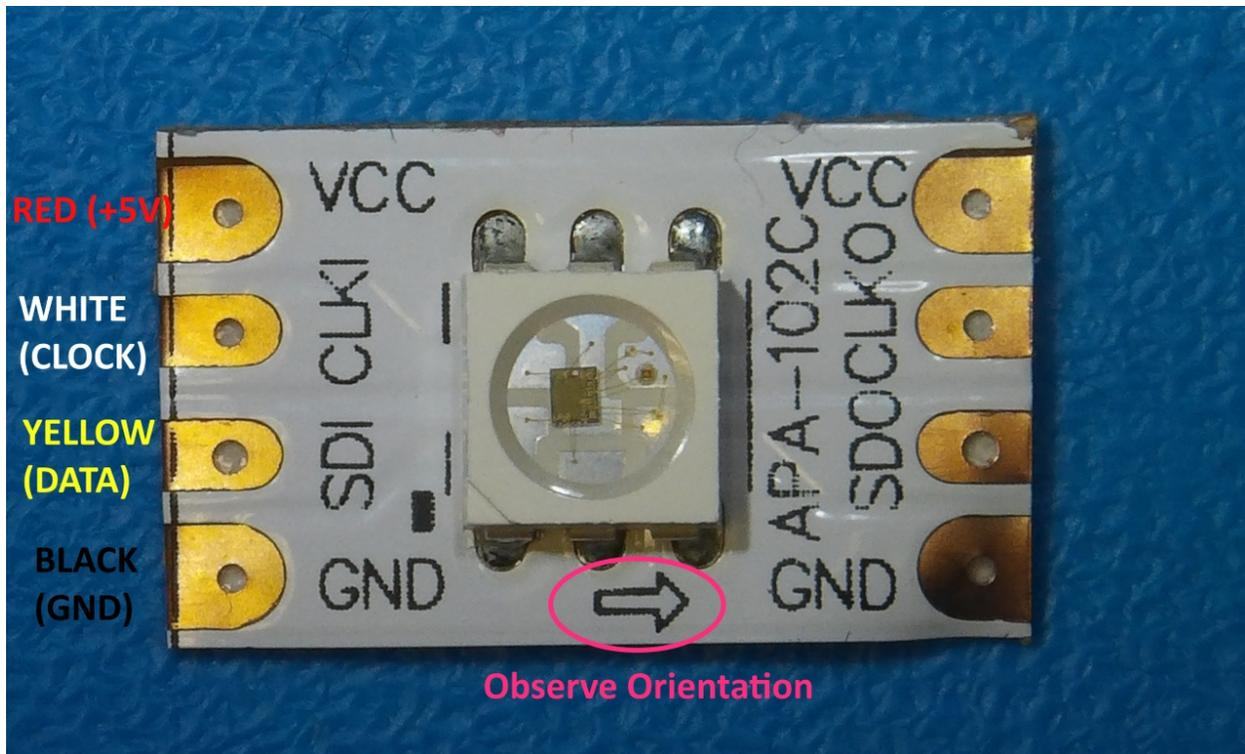
For an easy connection of the LED strip, it is recommended to connect four wires / leads to it, with a single pin socket, like the ones shown below. These wires can be obtained anywhere, and are sold -for example- as Raspberry PI jumper cables.
