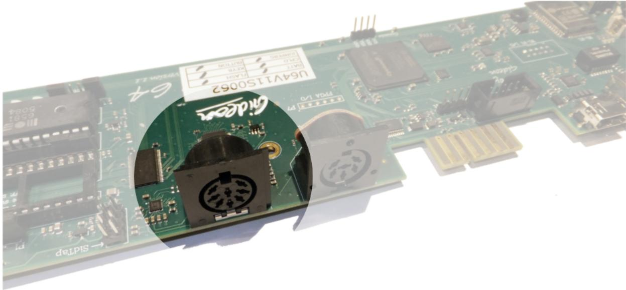
The 8-pin DIN ( audio/video ) connector can output several different video signals, for each type you need a special assembled cable.
